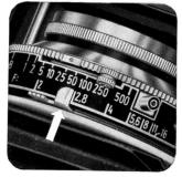
Exposure Time is set by turning the shutter speed ring, until the red dot is opposite the required speed. Figure "1" is one second; all the other figures are fractions of a second. — With the exception of \$^{1}\_{500}\$ second, all shutter speeds may be set after the shutter has been tensioned.
